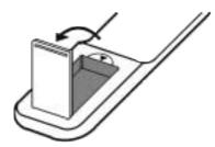
1 With your thumb nail, pull up the slit as indicated by the arrow to remove the battery cover.
